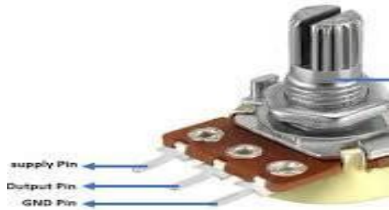
FIG 4 A 10KILOHM 5VOLTS ROTARY POTENTIOMETER.
