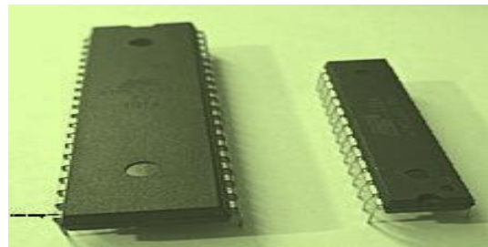
FIG 9 A MICRO CONTROLLER UNIT (ATMEGA 328p) DUAL IN-LINE PACKAGE (DIL) VERSION WITH 28 PINS
